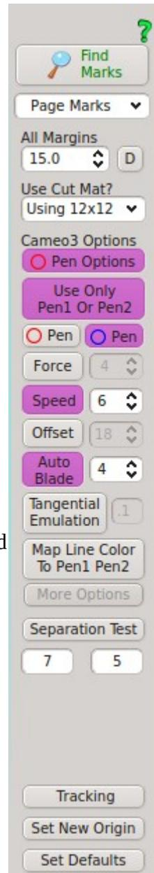
Tux Plot will only use the values for speed, pressure etc in the main Tux Plot window if using a Cameo or Cameo2. Enable red pen options are available to Cameo3 models only.
